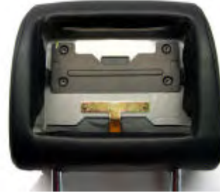
Headrest cushion with electronics mounting bracket installed
