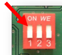
dip switches of tuner-box
