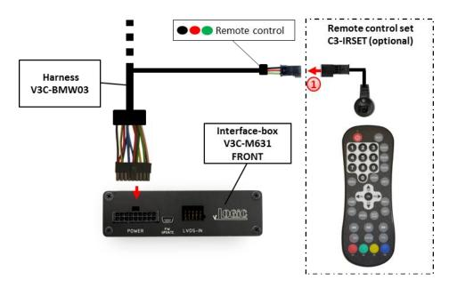
1 Connect the IR-sensor C3C-SENSOR to the female black/red/green 3pin AMP connector of harness V3C-BMW03 and locate the sensor in an accessible place.
