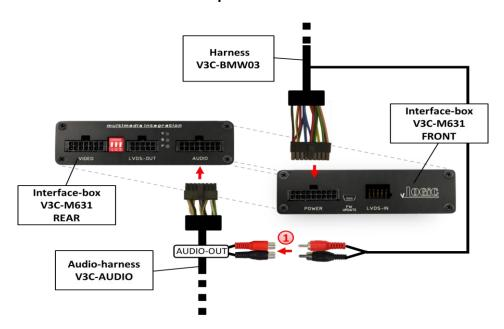
1 Connect the audio-RCA of harness V3C-BMW03 to the female RCA-connectors AUDIO OUT of the audio-harness V3C-AUDIO.
