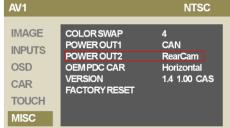
3 On some vehicles the reverse light signal doesn't exist on the CAN-bus. Connect the white wire of harness V3C-BMW03 to reverse light signal (+12V of reverse light) if the v.LOGiC doesn't switch to the rear-view camera automatically after the described OSD-setup (see next chapter).
