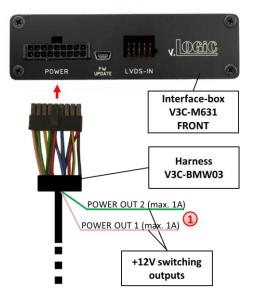
You can configure the both +12V trigger outputs separately. The pink wire is POWER OUT 1 and the green wire is POWER OUT 2.
