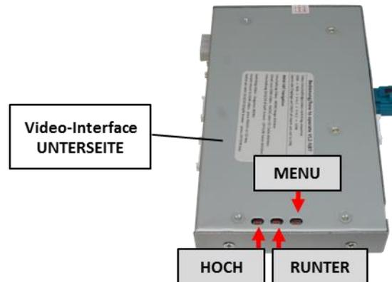
After installing the sources the picture settings can be changed using a pen on the buttons of the video interface. Press the MENU button to open settings menu on the OSD and to switch to the next setting. UP and DOWN change the corresponding values. The buttons are embedded in the housing to avoid accidental changes during or after installation.
