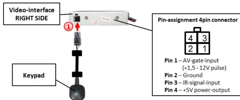
① Connect the female 4pin connector of the keypad to the male 4pin connector of the video-interface.
