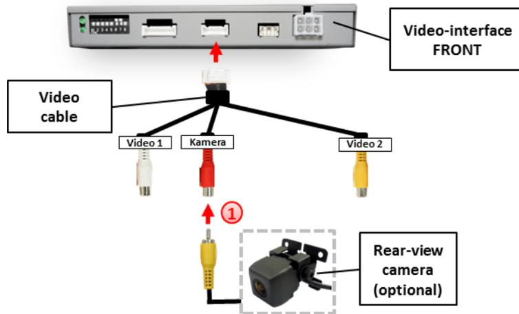
① Connect the video-RCA of the after-market rear-view camera to the female RCA port of the video-interface which is labeled as CAM.
