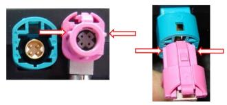
**Note:** The marked lug of the female 4pin HSD LVDS connector of the vehicle harness has to be cut off in some vehicles! The colour of the female 4pin HSD LVDS connector in vehicles with 8" monitor is grey.
