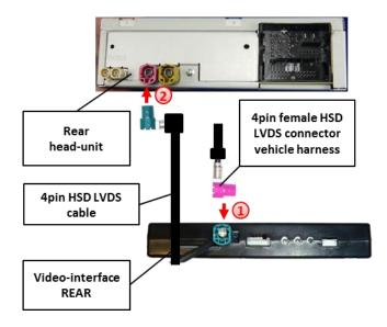
1 Remove female 4pin HSD LVDS connector from the rear of the head-unit and connect it to the male 4pin HSD LVDS connector of the video-interface.
