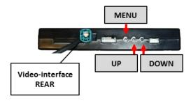
After installing the sources the picture settings can be changed using a pen on the buttons of the video interface. Press the MENU button to open settings menu on the OSD and to switch to the next setting. UP and DOWN change the corresponding values. The buttons are embedded in the housing to avoid accidental changes during or after installation.
