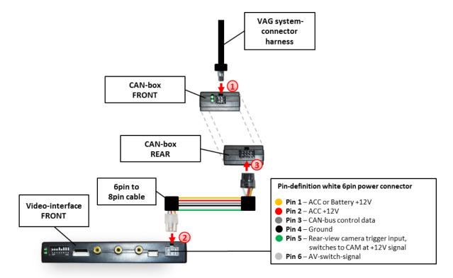
1 Connect black female 6pin Micro-Fit connector of the VAG system-connector harness to the male 6pin Micro-Fit connector of the CAN-box.
