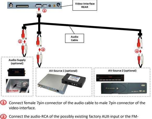
modulator to the female RCA port AV-Out of the audio cable.
