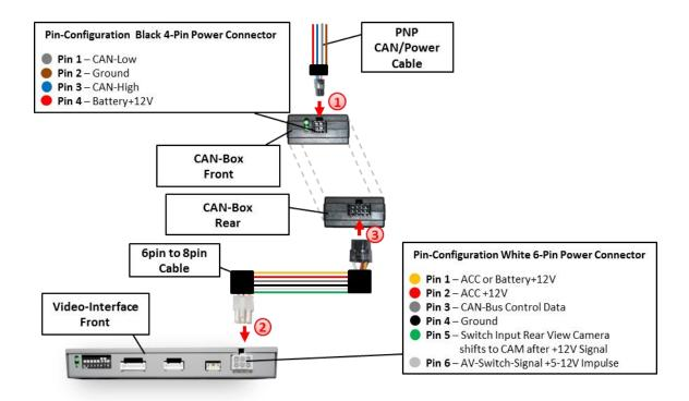
Connect black female 4pin Micro-Fit connector of PNP Can/Power Cable to the 4pin Micro-Fit connector of the CAN-box.
