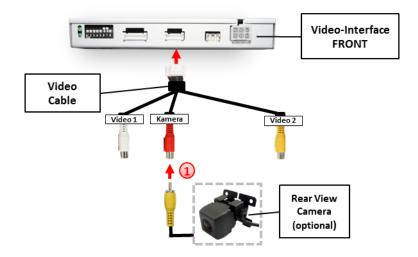
(1) Connect the video-RCA of the after-market rear-view camera to the female RCA port of the video-interface which is labeled as CAM.
