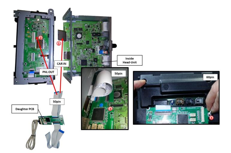
Disconnect optical laeds housed between mainboard of Head-Unit and monitorpanel. Connect flex-wire CAR-IN of daughter PCB to flex-wire base of the mainboard's Head-Unit. For this procedure you may either use the original flex-wire or the flexwire of daughter PCB.
