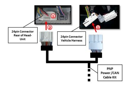
Disconnect the 24pin Connector of Vehicle harness at the rear of Head-Unit and connect it to the 24pin Connector of PNP Power/CAN Cable Kit.
