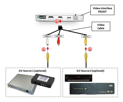
Connect 6pin male connector of video cable to female 6pin connector of videointerface
