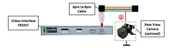
(1) Additionally, the +12V (max. 500mA) power supply for the rear-view camera can be taken from the green wire of the 6pin to 8pin cable.
