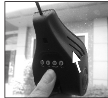
6. If need to take down the car black box , just hold it and push up.
