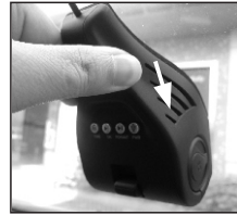
3. Push the car black box after put it into the holder correctly
