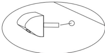
Put the cable and the thread through the hole and fasten the camera with its ring and screw nut.
