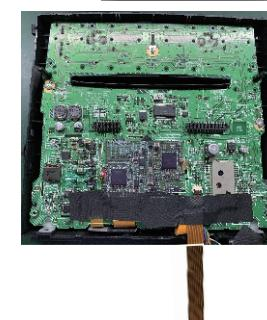
3) Cover the FPC cable with tape and install the original panel, then connect the FPC extension cable to the adapter plate as shown in the picture above.
