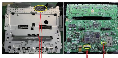
1) Separate the removed host and the panel, stick the protective tape at the position shown in the figure, and open the 30PIN wiring and 4PIN touch wiring of the display.
