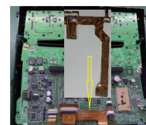
2) Take out the FPC cable as shown and install it as required to avoid short circuit
