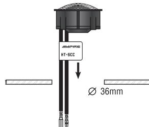
Install the tweeters like shown. Then connect the tweeter cables to the terminals of the FWHT-SCC crossover. Connect the crossover input wires (silver-blue = plus, silver = minus) to your headunit or amplifier. Be sure of right connections.
