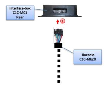
1 Plug harness C1C-ME20 into 12pin Molex of Interface-box C1C-M01.
