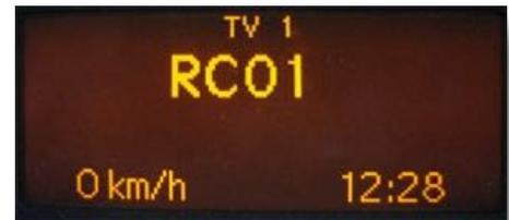
If the vehicle has no MFD display in the instrument panel, you must count the notches when turning the knob (to the right +1, to the left -1). At the same time, remember that the starting point is channel RC01 (the first notch to the right is then already RC02).
