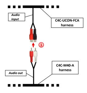
Connect the audio cinch sockets "Audio input" of the C4C-UCON-FCA harness to the audio cinch plugs "Audio out" of the C4C-M40-A harness.
