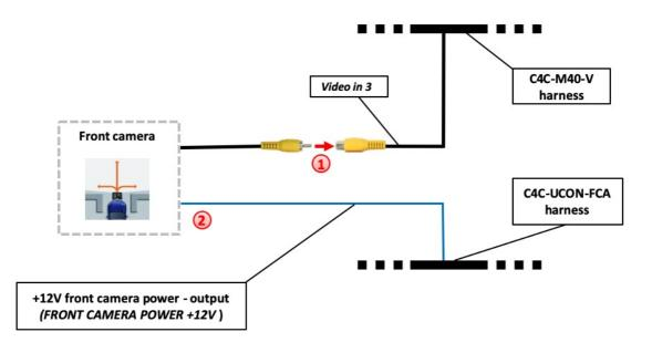
Connect the video RCA of the after market front camera to the female RCA connector "Video in 3" of harness C4C-M40-V.
