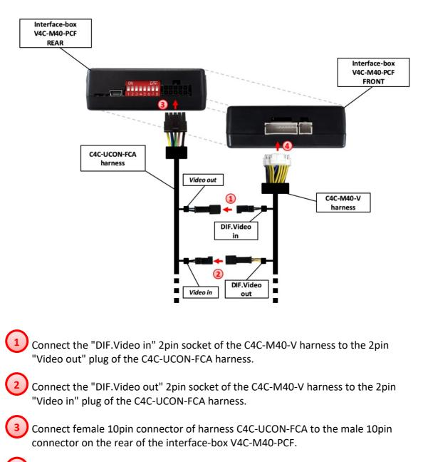
Connect female 18pin connector of harness C4C-M40-V to the male 18pin connector on the front of the interface-box V4C-M40-PCF.
