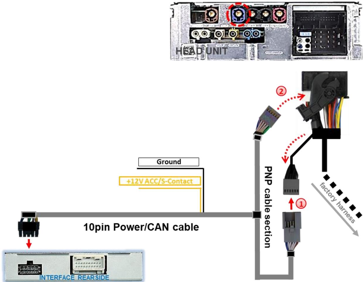
① Remove the female Quadlock connector of the vehicle harness from the rear-side of the head-unit and connect the previously clipped out black female 12pin connector (see graphic) to the male 12pin connector of the PNP harness.
