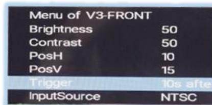
**“Delay”-function for front camera.** The **“delay”** setting determines the automatic switching to front camera input after reverse gear is disengaged, as well as its display duration on the display. Adjustable values are 5s after REV, 10s after REV, 15s after REV, 20s after REV are.
