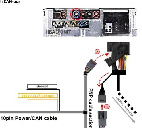
Remove the female Quadlock connector of the vehicle harness from the rear-side of the headunit and connect the previously clipped out black female 12pin connector (see graphic) to the male 12pin connector of the
