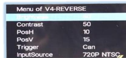
**„CAN”-function with CAN-bus connection.** With **„CAN”** setting, on engagement of reverse gear, the interface switches automatically to **V4-Reverse/HDMI\*** for a CVBS/AHD rear-view camera. Requirement is, that the reverse gear signal is recognised by the interface from vehicle CAN-bus.
