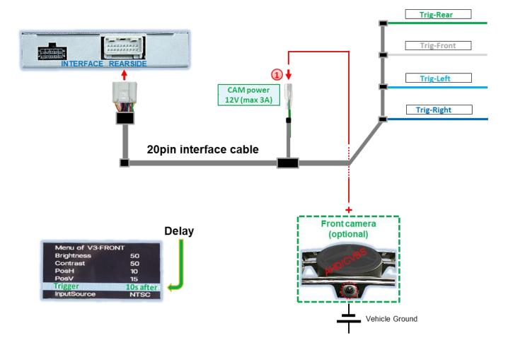
The green wire CAM power 12V (max 3A) can be used to supply power to front camera (and all other cameras connected to the video inputs), as it only carries current for the duration of any camera activation (some cameras are not continuously current-stable). Requirement is dip 3 = ON (black 8dip switch bench). Then green wire carries +12V (max 3A) as power supply for the front camera as long as the front camera input is displayed.
