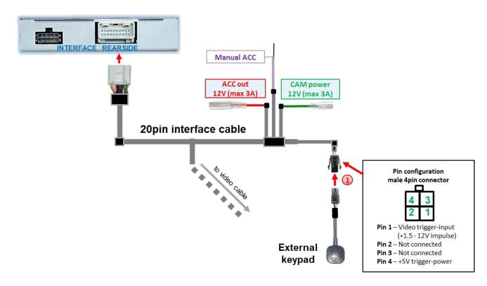
① Connect female 4pin connector of keypad to male 4pin connector of 20pin interface cable.
