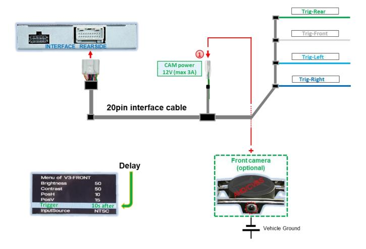
The green wire CAM power 12V (max 3A) can be used to supply power to front camera (and all other cameras connected to the video inputs), as it only carries current for the duration of any camera activation (some cameras are not continuously current-stable). Requirement is dip 3 = ON (black 8dip switch bench). Then green wire carries +12V (max 3A) as power supply for the front camera as long as the front camera input is displayed.
