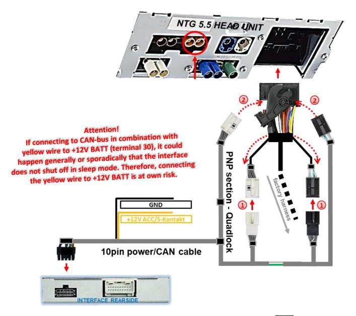
Remove the female Quadlock connector of the vehicle harness at the rear-side of the head-unit and connect the previously clipped out white and black female 12pin connectors to the white and black male 12pin connectors of the PNP harness (see graphic).
