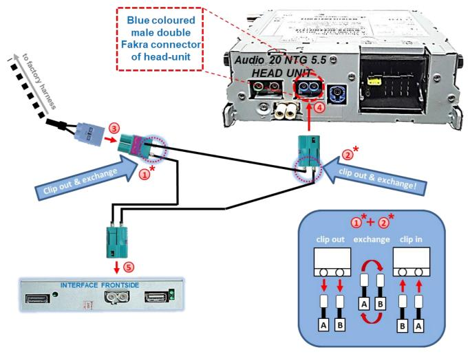
Unlock the picture signal cable's green male double Fakra connector's locking mechanism, clip out both cables to exchange them (see the blue diagram), clip in the exchanged cables and again lock the connectors locking mechanism.
