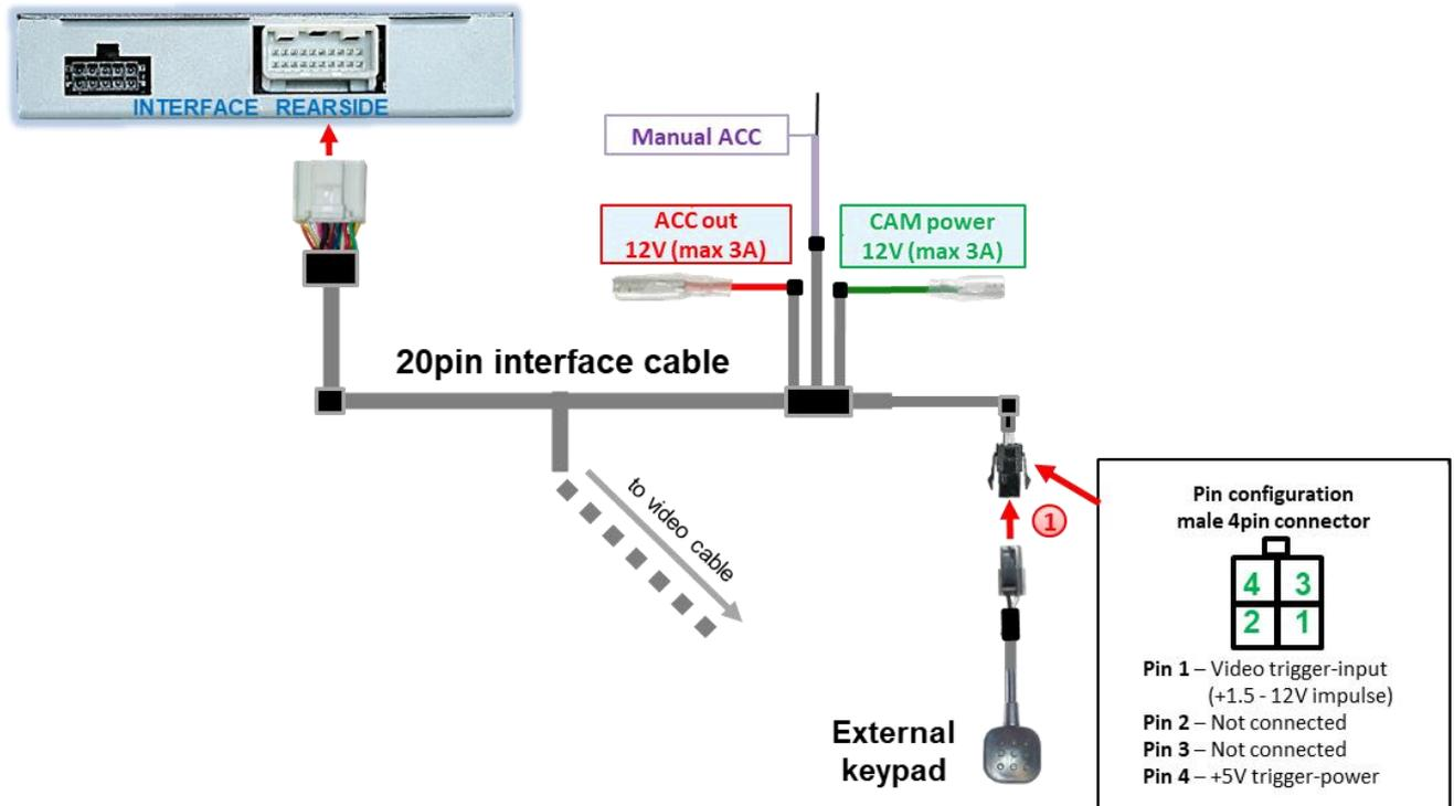
1 Connect female 4pin connector of keypad to male 4pin connector of 20pin interface cable.
