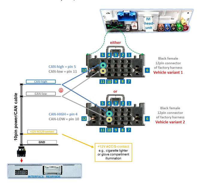
Connect blue CAN-high wire and grey CAN-low wire of 10pin power/CAN cable to corresponding chambers of black female 12pin connector of vehicle harness. There are two known vehicle pin definition variants displayed above.
