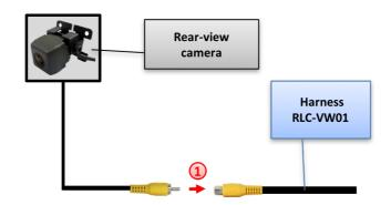
Connect the video RCA of the after-market rear-view camera to female RCA connector of harness RLC-VW01.
