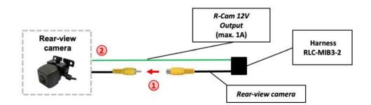
Connect the video RCA of the rear-view camera to the female RCA connector with the label *"Rear-view camera"* of RLC-MIB3-2 harness.
