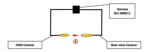
If there is a factory rear-view camera installed, connect the male RCA plug with the label "OEM Camera" to the female RCA connector with the label "Rear-view Camera" from RLC-POR03-2 harness.
