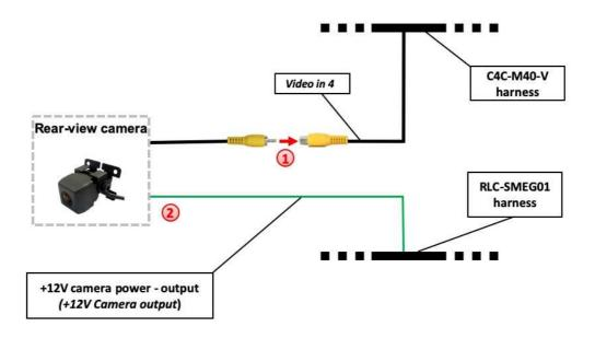
Connect the video RCA of the after market rear-view camera to the female RCA connector "Video in 4" of harness C4C-M40-V.
