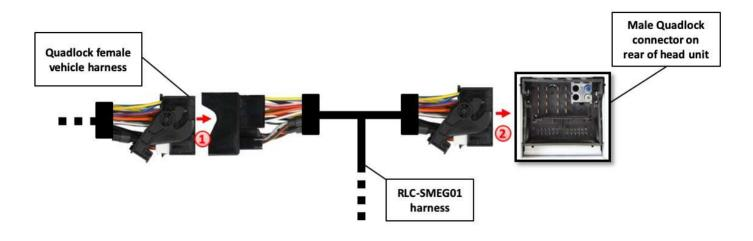
1 Transfer Quadlock connector of vehicle harness from rear of the head unit into male Quadlock connector of harness RLC-SMEG01.
