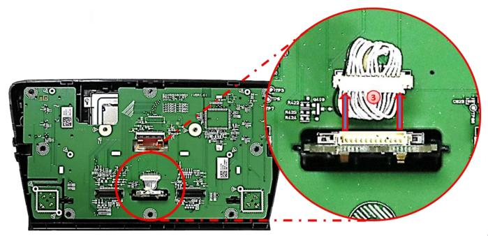
3 Disconnect the female 12pin connector from its 12pin SD card connector (keep connected at mainboard).
