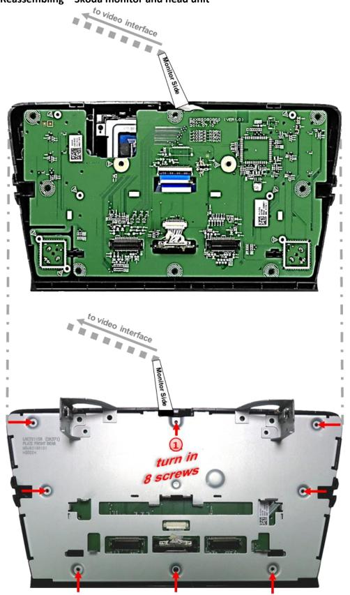
Lead the picture signal cable out at an appropriate location and reassemble the monitor's rear housing part by using the 8 screws.
