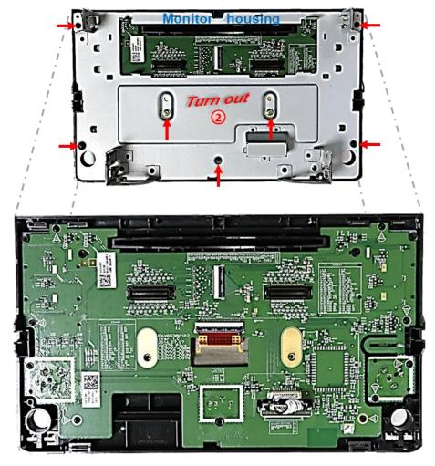
2 Turn out the 7 screws (red arrows) at the rear side of the monitor and remove the metal sheet to set free the mainboard's ribbon cable base with the factory picture signal cable.
