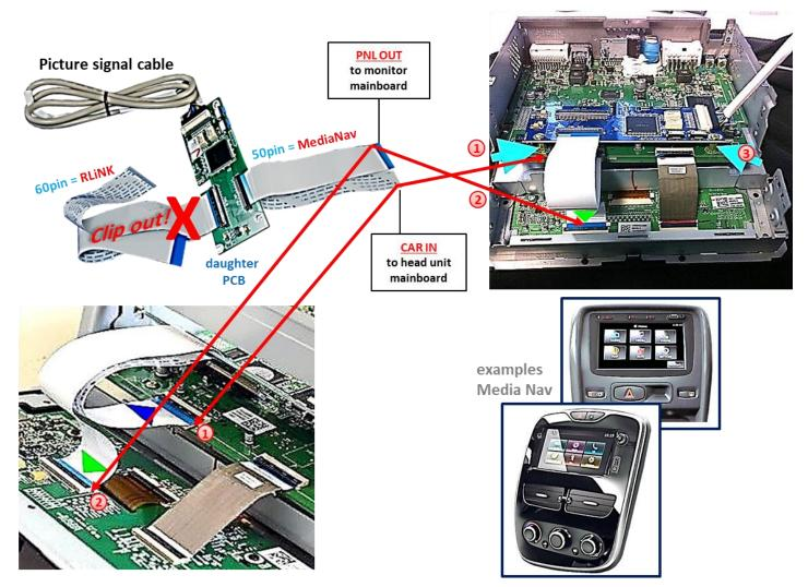
Disconnect the optical leads housed between the monitor's mainboard and the monitorpanel. Connect the daughter PCB's ribbon cable CAR-IN to the ribbon cable base of the monitor's mainboard. For this procedure you may either use the original ribbon cable or the ribbon cable of the daughter PCB. Make sure that the connector pins of each pin connector are faced to the platinum before clipping them.
