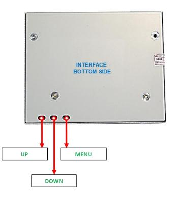
The picture settings are adjusted by the 3 buttons on the video-interface. Press the MENU button to open the OSD settings menu or to switch to the next menu item. Press UP and DOWN change the selected value. The buttons are embedded in the housing to avoid accidental changes during or after installation. Picture settings must be done separately for RGB, AV1, AV2 and CAM while the corresponding input is selected and visible on the monitor.
