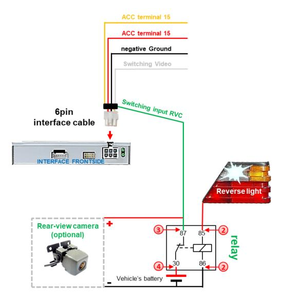
Connect the green switching input cable to the output connector (87) of the relay.
