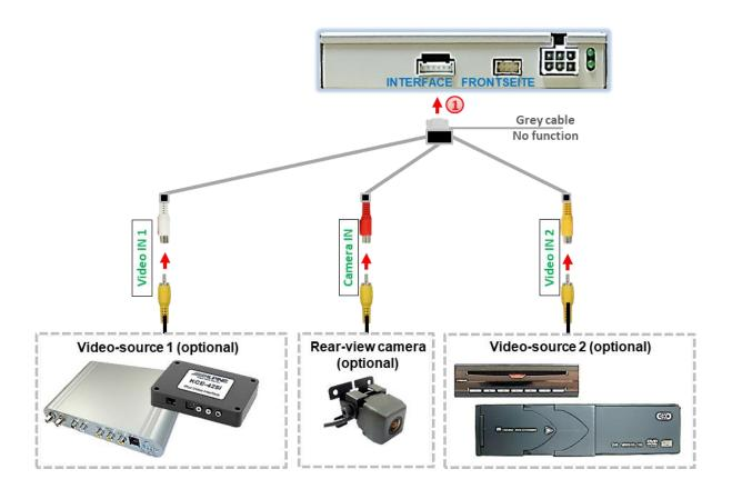
Connect the 6pin connector of the video cable to the 6pin connector of the video interface.
