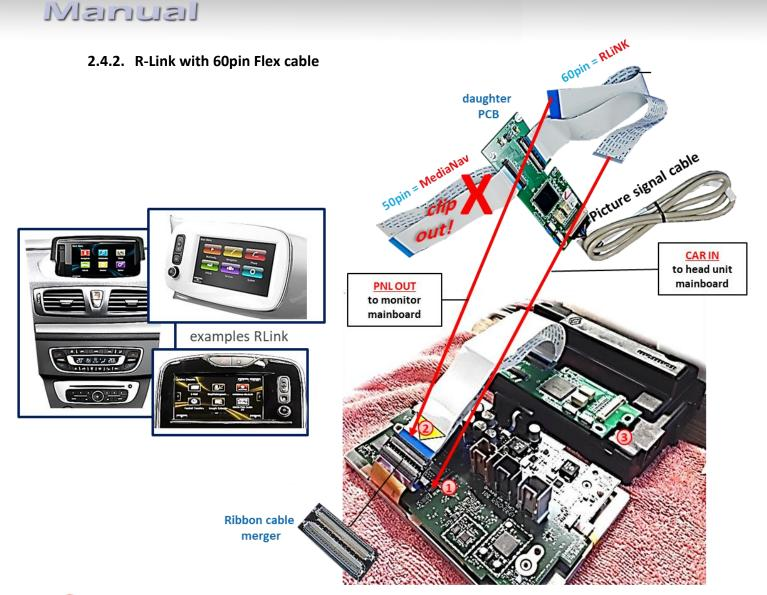
Remove the Ribbon cable between the monitor's monitor panel and the monitor PCB. Connect the daughter PCB's ribbon cable CAR-IN to the ribbon cable base of the main PCB. For this procedure you may either use the original ribbon cable or the ribbon cable of daughter PCB. Make sure that the connector pins of each pin connector are faced to the platinum before clipping them.
