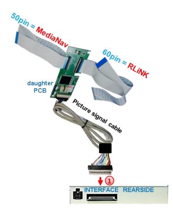
Connect the female 20pin connector of the daughter PCB to the male20pin connector of the picture signal cable and connect the second male 20pin connector opposite the cable to the female 20pin connector of the interface. Take care for installing the cable in the right direction as both connectors seem to be identical. (Take notice of the wire's caption "MONITOR SIDE" and "BOX SIDE"
