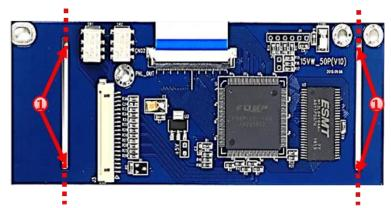
Carefully, sever the 4 predetermined breaking points of the daughter PCB and remove both side parts.
