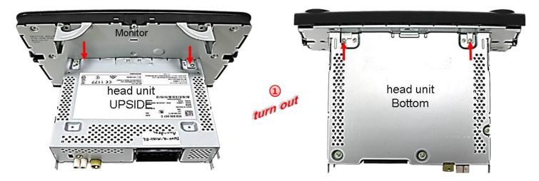
1 Turn out both screws at the **outer** side of the top part of the head unit (red arrows) and both screws at the bottom part of the head unit (red arrows). Separate the head unit from the monitor and lay it aside.
