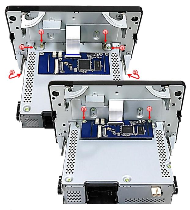
(1) Carefully, plug the head unit into the monitor again and fix it with the 4 screws on its top and its bottom.
