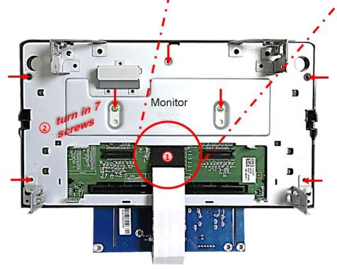
2 Fix the monitor's rear metal sheet by using the 7 screws.
