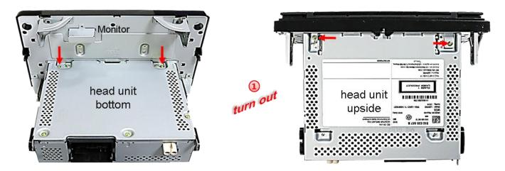
1 Turn out both screws at the **outer** side of the top part of the head unit (red arrows) and both screws at the bottom part of the head unit (red arrows). Remove the head unit from the monitor and lay it aside.
