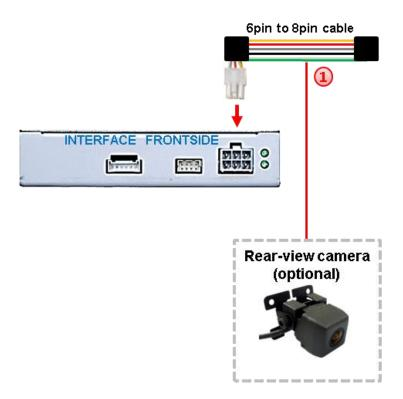
Additionally, the +12V (max. 500mA) power supply for the rear-view camera can be taken from the green wire of the 6pin to 8pin cable.
