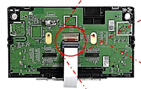
3 To avoid any kind of vibration-caused short circuits after the connection, it's necessary to isolate both sides of the merger with some kind of smooth issue tape as shown in the picture beside.
