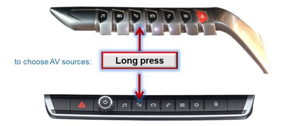
A long press of the infotainment's "Navi"-button switches the input from factory mode to the inserted video sources. If, by dip switch setting, all inputs are enabled, the order is the following:
