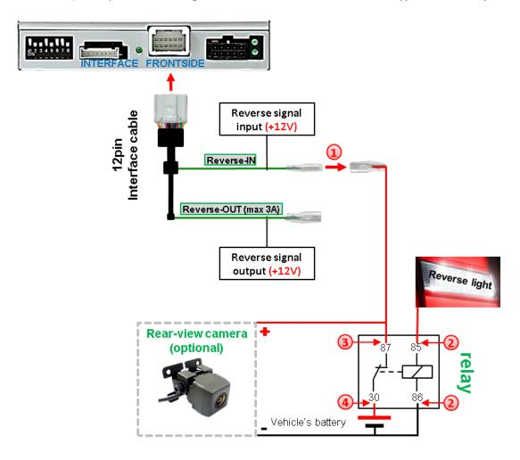
Disconnect the green cable's pre-connected male- and female connectors of the 20pin cable and connect the green input cable "Reverse-IN" to the output connector (87) of the relay.
