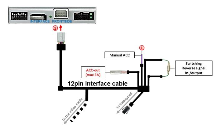
Connect the 12pin interface cable's purple coloured wire Manual ACC to +12V Ignition power or to +12V S-contact terminal 86s +12V (e.g. glove compartment illumination).
