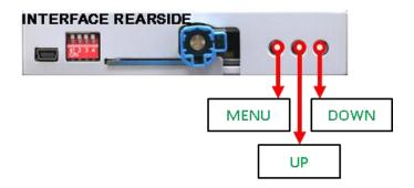
The picture settings can be adjusted by the 3 buttons on the video-interface. Press the MENU button to open the OSD settings menu. To switch to the next menu item, pressing UP and DOWN will change the selected value. The buttons are embedded in the housing to avoid accidental changes during or after installation. The picture settings have to be done separately for AV1 and AV2 while the corresponding input is selected and visible on the monitor.
