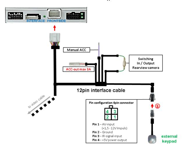
1 Connect the keypad's female 4pin connector to the video-interface's male 4pin connector.
