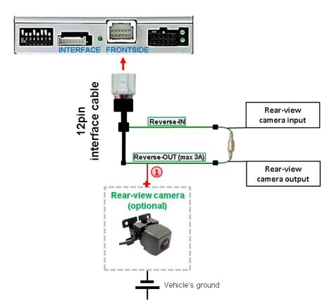
1 The 12 V power supply for the rear-view camera (max 3A) has to be taken from the green wire of the 20pin cable to avoid an unnecessary, permanent power supply to the camera electronic.
