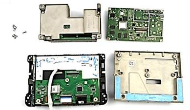
Carefully seperate the metal sheet that covers the monitor PCB.
