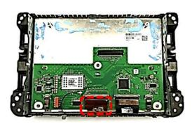
Clip out and disconnect the monitor's 60pin ribbon cable which has to be connected to the daughter PCB's ribbon cable base "OUT".
