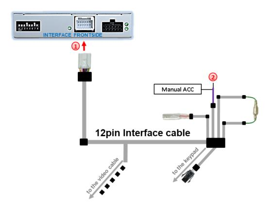
Connect the 12pin interface cable's white coloured female 12pin connector to the 12pin connector of the video interface.
