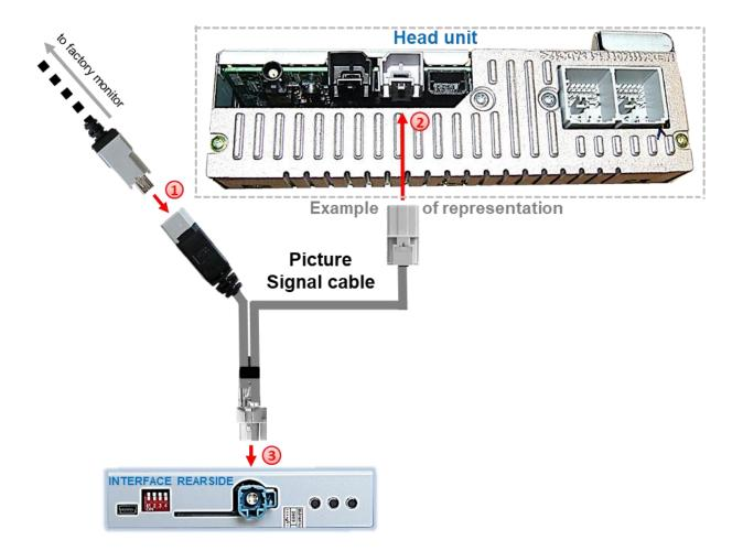
Disconnect the factory picture signal cable's male Mini USB connector at the rear-side of the head unit and connect it to the female Mini USB connector of the enclosed picture signal cable.
