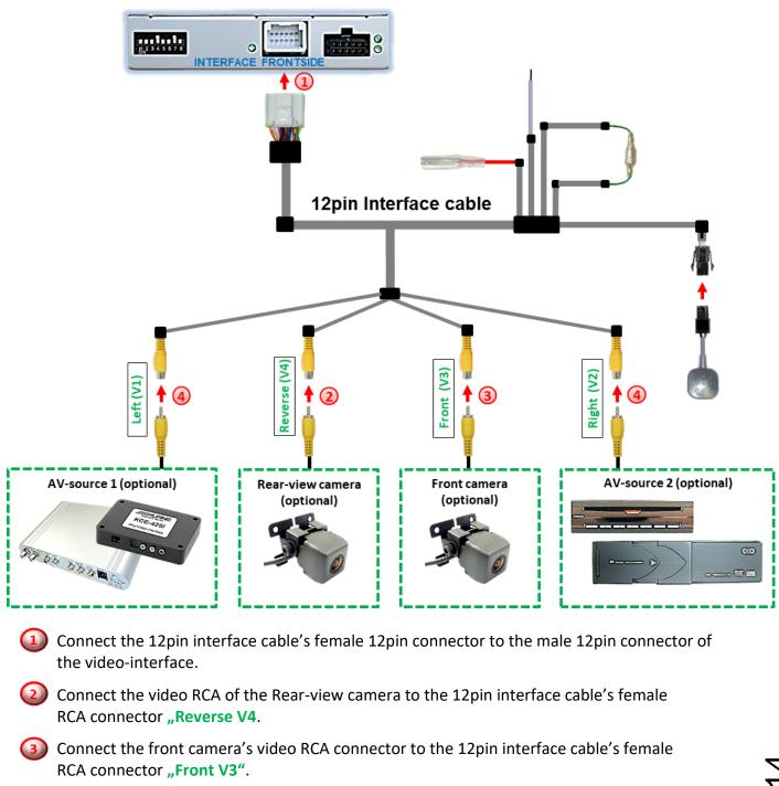
Connect the video RCA of the AV source 1 and 2 to the 12pin interface cable's female RCA connector "Left (V1)" and "Right (V2)".
