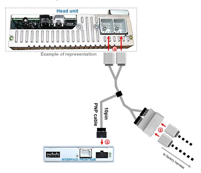
Connect the 10pin PNP cable's female 10pin connector to the 10pin connector of the video interface.
