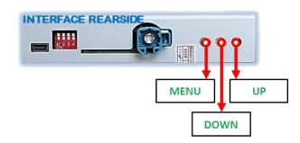
The picture settings are adjustable by the 3 push-buttons at the rear-side of the videointerface. Press the MENU button to open the OSD settings menu or to switch to the next menu item. Press UP and DOWN to change the selected value. The buttons are placed inside in the housing to avoid accidental changes during or after the installation. Picture settings must be done separately for all video inputs while the corresponding input is selected and visible on the monitor.
