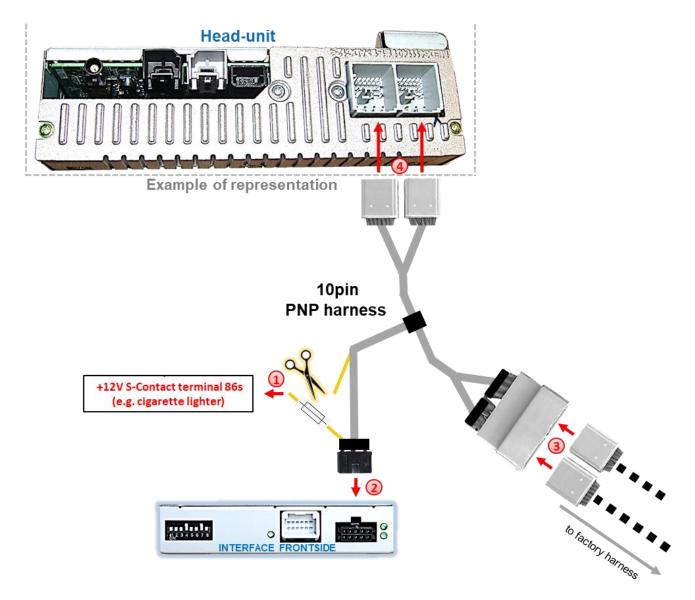
Cut the yellow wire of the PNP harness near the 10pin connector and connect it to the vehicle's +12V S-contact terminal 86s (e.g. cigarette lighter) Insulate the other side of the yellow cable, as it is powerded!
