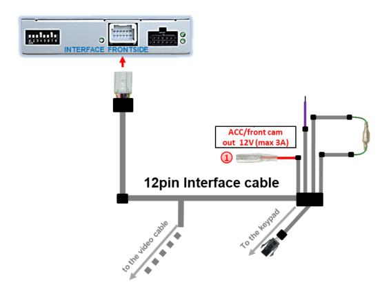
The red power supply output ACC/front cam out 12V (max 3A) can be used to power an external source and has a different assignment depending on the position of dip switch 1 (of the black 8 dips):
