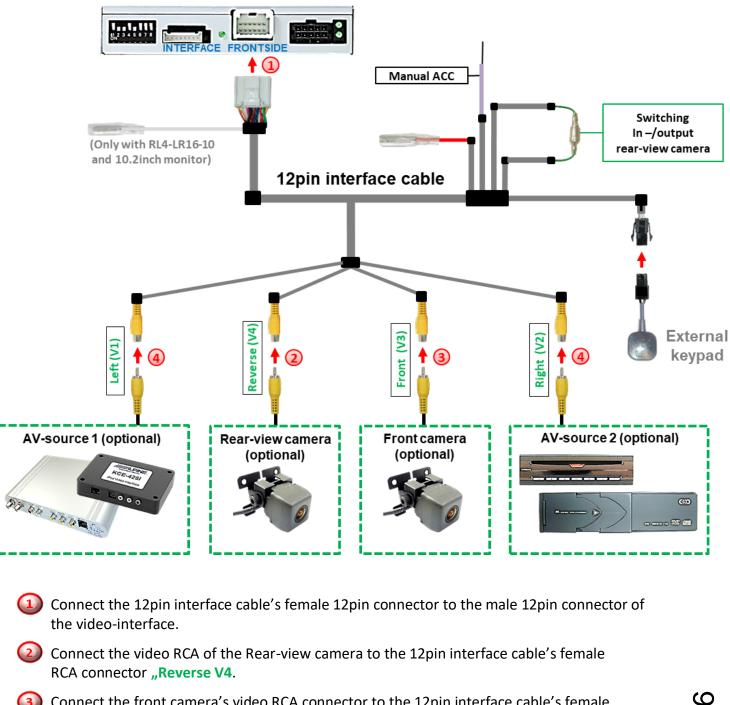
Connect the front camera's video RCA connector to the 12pin interface cable's female RCA connector "Front V3".
