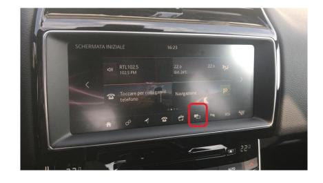
\* Non-compatible dual-view monitors can be recognised by the dual-view button:
