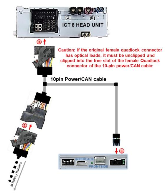
Connect the female 10pin connector of the 10pin Power / CAN cable to the 10pin connector of the video interface.
