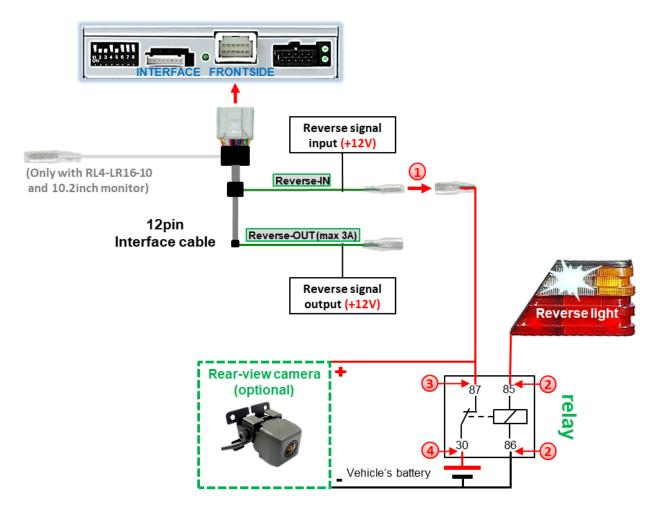
Disconnect the green cable's preconnected male- and female connectors of the 12pin interface cable and connect the green input cable "Reverse-IN" to the output connector (87) of the relay.
