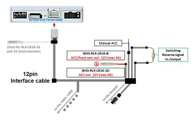
On the RL4-LR16-10, the red power supply output ACC out 12V (max 3A) can be used to power up an external source (independent of Dip-1 switch setting).
