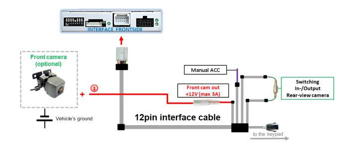
The red power supply output ACC/front cam out 12V (max 3A) can be used to power a front camera. If Dip 1 is set to ON (of the black 8 dips), the power supply output supplies +12V (max 3A) when the reverse gear is engaged and additionally 10 seconds delay after the reverse gear is disengaged.
