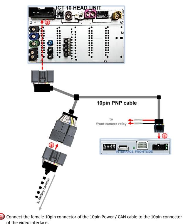
2 Remove the female 24pin connector of the vehicle harness from the rear-side of the head-
