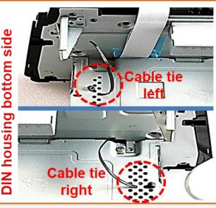
Pass a cable tie through on the right and left for subsequent attachment of the daughter PCB at the same points as shown in the picture.
