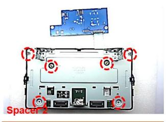
Close the monitor housing with the metal bracket and fix it with 4 of the original screws at the edges. The 2 enclosed spacers have to be screwed in the 2 free middle holes for the daughter PCB's fixing.
