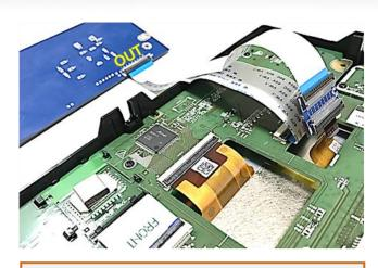
Connect the previously become free copper coloured factory ribbon cable to the merger of the daughter PCB's ribbon cable "OUT".
