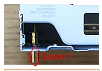
For later attachment of the daughter PCB to the Head Unit, mount one of the spacers supplied on the outside and fix it on the inside at the position shown. **See also Fig. 5**
