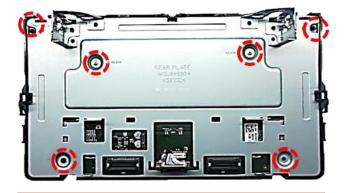
Screw out the 6 fixing screws at the monitor's backside and remove the metal bracket
