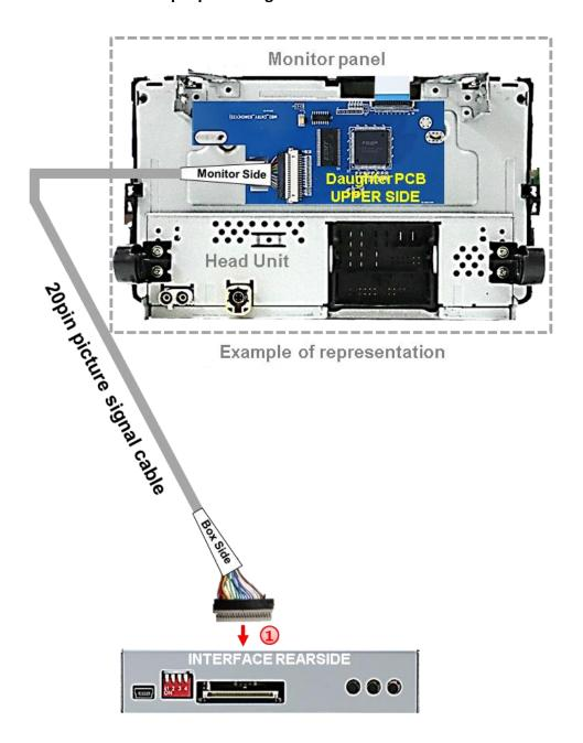
Connect the female 20pin connector of the daughter PCB's pre-connected 20pin picture signal cable to the video interface's male 20pin connector.
