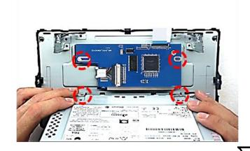
Fix the PCB with 2 screws. Fix the monitor with installed PCB to the head unit with the screws at the upper and the bottom side of the head unit.
