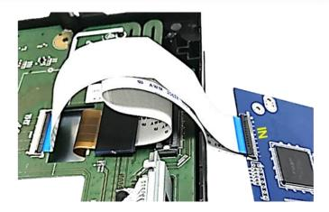
Connect the daughter PCB's ribbon cable "IN" to the previously become free monitor PCB's ribbon cable base.
