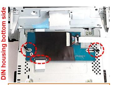
Pass the two ribbon cables under the daughter PCB, connect them to the daughter PCB's two ribbon cable bases and fix the daughter PCB in place.
