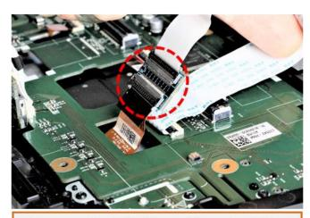
After connecting both ribbon cables, protect ribbon cable merger and ribbon cables from short circuits or cable damage with tape when leading them out before reassembling the monitor panel.
