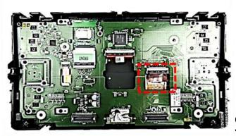
After removing the metal bracket, gently disconnect the factory picture signal cable at the monitor PCB's ribbon cable base.
