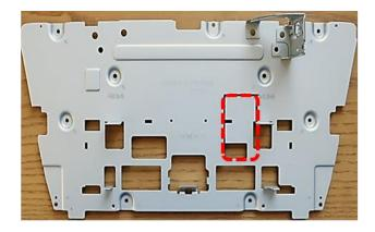
Remove the head unit from the monitor (see VW/Seat). For later leading-out the ribbon cables, cut out the monitor back plate at the marked point and protect the cut edges with fabric tape.
