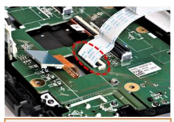
Clip the second enclosed ribbon cable to the previously become free ribbon cable base of the monitor board with the contacts facing upwards.
