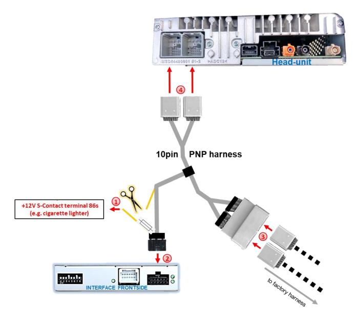
1 Cut the yellow wire of the PNP harness near the 10pin connector and connect it to the vehicle's +12V S-Contact (terminal 86s). Insulate the other side of the yellow cable, as it is powered!
