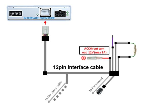
1 The red power supply output ACC/front cam out 12V (max 3A) can be used to power an external source and has a different assignment depending on the position of dip switch 1 (of the black 8 dips):
