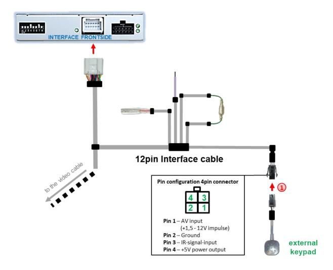
Connect the female 4pin connector of the keypad to the male 4pin connector of the 12pin interface cable.
