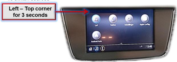
Switchover by vehicle buttons isn't possible in all vehicles. In some vehicles the external keypad has to be used.
