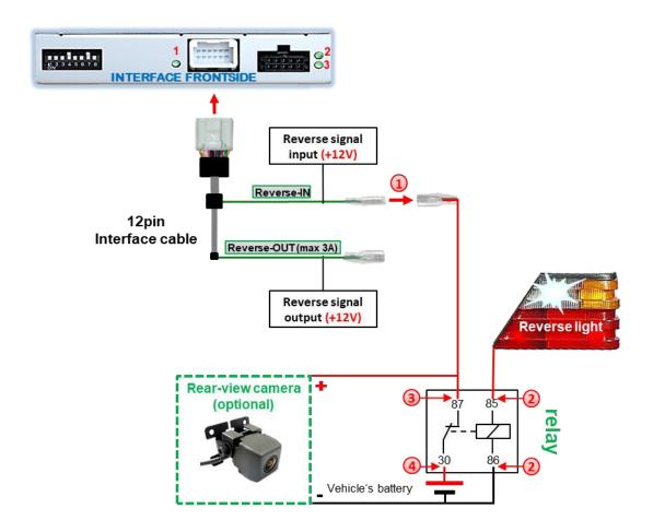
Disconnect the green cable's pre-connected male- and female connectors of the 20pin cable and connect the green input cable "Reverse-IN" to the output connector (87) of the relay.
