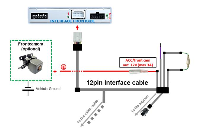
1 The red power supply output ACC/front cam out 12V (max 3A) can be used to power a front camera. If Dip 1 is set to ON (of the black 8 dips), the power supply output supplies +12V (max 3A) when the reverse gear is engaged and additionally 10 seconds delay after reverse gear is disengaged.
