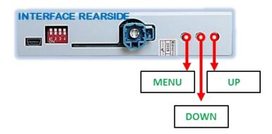
The picture settings can be adjusted by the 3 buttons on the video-interface. Press the MENU button to open the OSD settings menu. To switch to the next menu item, pressing UP and DOWN will change the selected value. The buttons are embedded in the housing to avoid accidental changes during or after installation. The picture settings have to be done separately for AV1 and AV2 while the corresponding input is selected and visible on the monitor.
