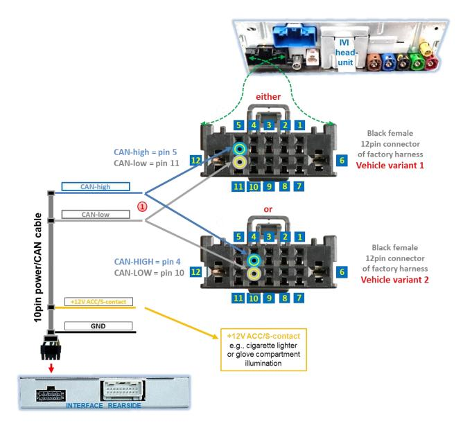
Connect blue CAN-high wire and grey CAN-low wire of 10pin power/CAN cable to corresponding chambers of black female 12pin connector of vehicle harness. There are two known vehicle pin definition variants displayed above.
