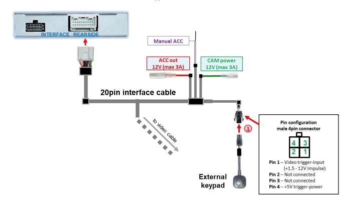
Connect female 4pin connector of keypad to male 4pin connector of 20pin interface cable.
