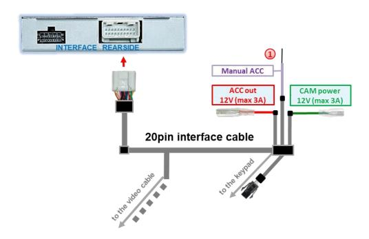
Connect purple wire Manual ACC of 20pin interface cable to +12V S-contact terminal 86s or ACC terminal 15r of vehicle (e.g., cigarette lighter, glove compartment illumination).
