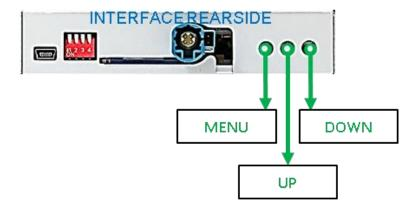
The picture settings are adjustable by the 3 push-buttons on the video-interface. Press the MENU button to open the OSD settings menu or to switch to the next menu item. Press UP and DOWN to change the selected value. The buttons are placed inside in the housing to avoid accidental changes during or after the installation. Picture settings must be done separately for Video1 and Video2 while the corresponding input is selected and visible on the monitor.
