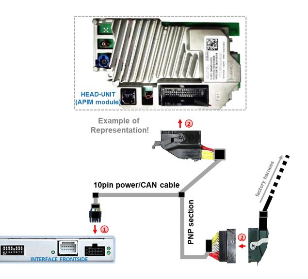
Connect the 10pin power/CAN cable's female 10pin connector to the 10pin connector of the video interface.
