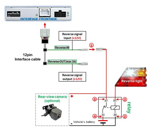
Disconnect the green cable's preconnected male- and female connectors of the 12pin interface cable and connect the green input cable "Reverse-IN" to the output connector (87) of the relay.
