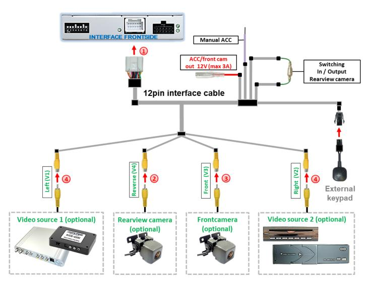
Connect the 12pin interface cable's female 12pin connector to the male 12pin connector of the video-interface.
