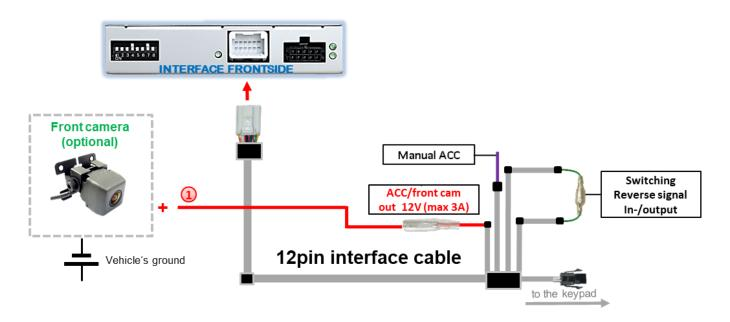
The red power supply output Front cam out +12V (max 3A) can be used to power a front camera. If Dip 1 is set to ON (black 8 dips), the power supply output gives +12V (max 3A) when reverse gear is engaged
