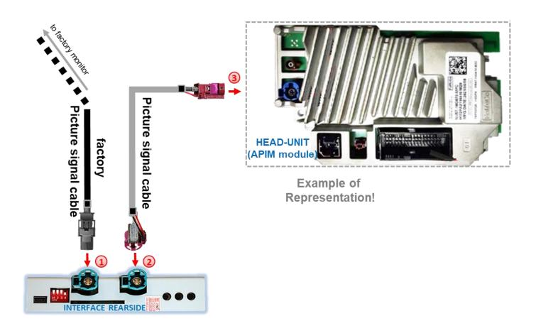
Disconnect the female HSD+2 connector (colours may vary) at the rear-side of the head unit (APIM module) and connect it to the waterblue coloured male HSD+2 connector **"TO LCD"** of the video interface.
