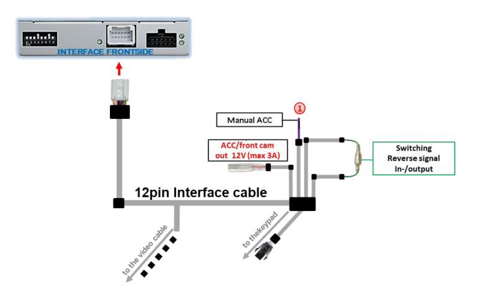
If, after connecting the PNP harness, no interface LED lightens up while the ignition is turned on, the purple coloured wire Manual ACC of the 12pin interface cable has to be connected additionately to ACC or S-contact terminal 86s +12V (e.g. glove compartment illumination).
