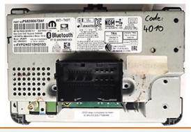
Remove the screws and open the head-unit. Remove the main board, the metal plates, the monitor board and the plastic housing.
