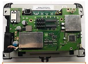
Reassemble the head-unit mainboard after carefully routing out the 20pin picture signal cable. .
