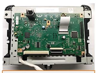
After the 40pin ribbon cable has been led out at the indicated point, mount the monitor board again and clip the 40pin ribbon cable to the ribbon cable base of the mainboard.
