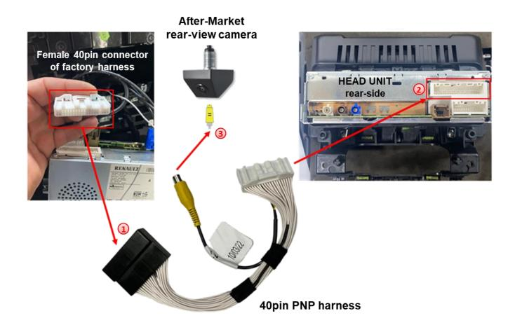
Disonnect the female 40pin connector of the factory harness at the rear-side of the headunit and connect it to the male 40pin connector of the 40pin PNP cable.
