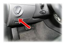
When the navigation has booted, connect the TF-MMI2G interface to the OBD-socket for about 15 seconds in order to activate the function. Disconnect the TF-MMI2G from the OBD-socket.
