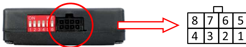
Pin-assignment male 8pin connector of TV-500
