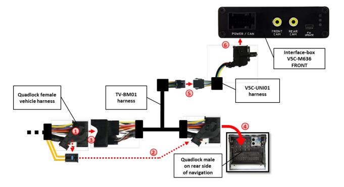
Remove the female Quadlock connector of the vehicle harness from the rear of the navigation computer.
