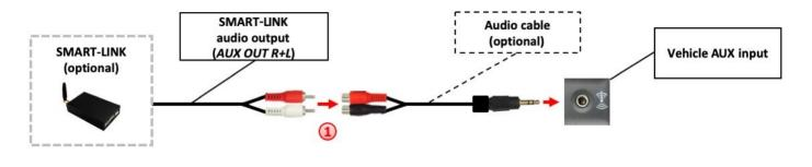
By using an audio cable (sold separately), connect the audio output of the SMART-LINK module to the vehicle AUX input.
