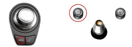
In **BMW** in the vehicle's **Entertainment** menu activate **AUX** and in **Mini** in the vehicle's **CD/Multimedia** menu, activate **AUX front** by iDrive and after it **long press MENU** button (1- and 2-button iDrive + Mini) to choose the interface as current AV-source.
