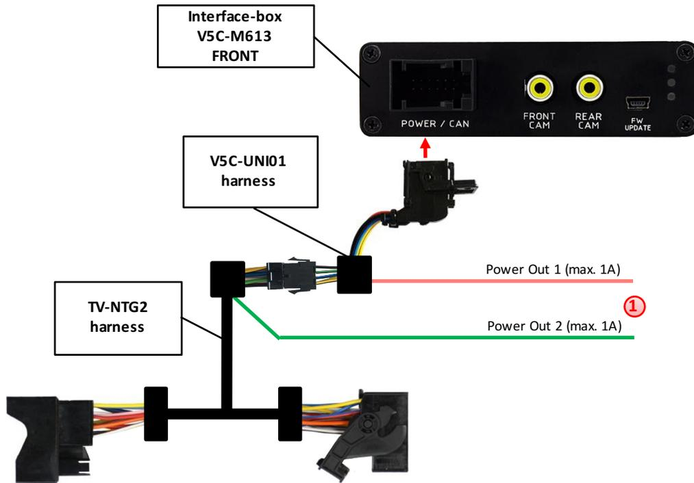
**1** You can configure the both +12V trigger outputs separately. The pink wire is POWER OUT 1 and the green wire is POWER OUT 2.
