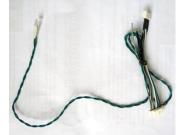
■ When the installer use the IR-RGB or IR\_DVD without carrier frequency, he needs to connect the IR output wire to the ir-sensor's signal wire.[all ir-sensors have 3 wires inside, +5V,GND, and signal]
