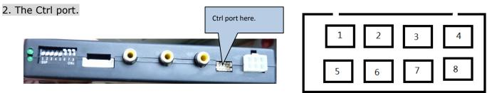
The Ctrl port has 8 pins, it is not necessary for the installers to
