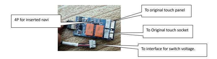
When the touch screen is not used for navigation, it can also be used for DVD/TV control for installed device.
