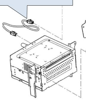
Then the interface's LVDS tail plug should be inserted onto this monitor's rear socket. Which was used by CD's 4Pin connector.
