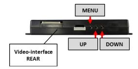
After installing the sources the picture settings can be changed using a pen on the buttons of the video interface. Press the MENU button to open settings menu on the OSD and to switch to the next setting. UP and DOWN change the corresponding values. The buttons are embedded in the housing to avoid accidental changes during or after installation.
