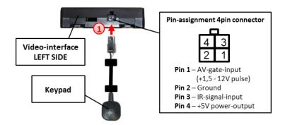
Connect the female 4pin connector of the keypad to the male 4pin connector of the video-interface.
