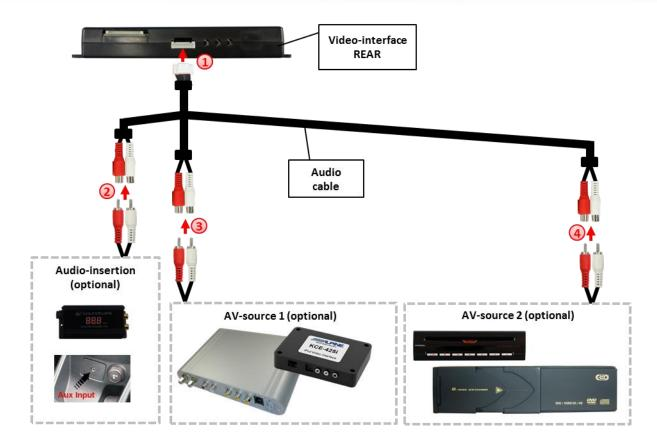
**Note:** If only one AV-source shall be connected, it is possible to connect the video output of the AV-source to video IN1 of the video-interface and the audio output of the AV-source direct to the audio-insertion.
