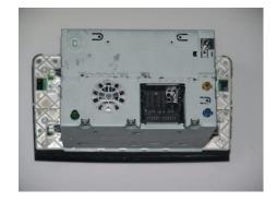
Remove the upper cover including the DVD/ navigation device. The external daughter PCB is plugged in between the flex cable of the monitor panel and the mainboard of the head-unit.
