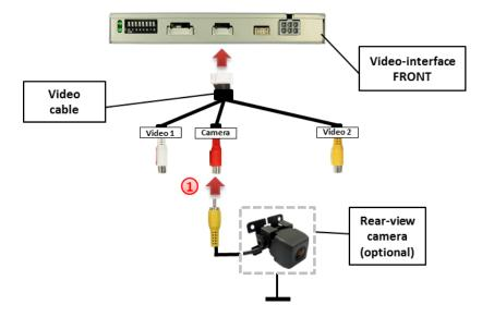
1 Connect the video-RCA of the after-market rear-view camera to the female RCA port of the video-interface which is labeled as CAM.
