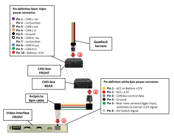
1 Connect black female 10pin Micro-Fit connector of the Quadlock harness to the male 10pin Micro-Fit connector of the CAN-box.
