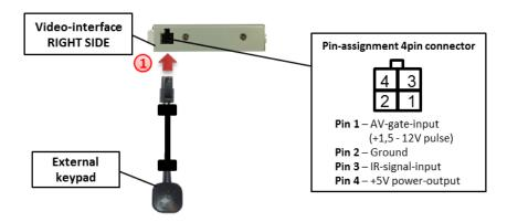
1 Connect the female 4pin connector of the keypad to the male 4pin connector of the video-interface.
