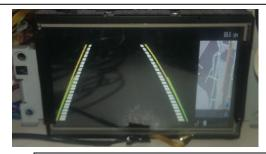
The "Guide CTRL.....ON": the installer can set ON/OFF to enable the parking guide line, which shows the safe zone when parking.
