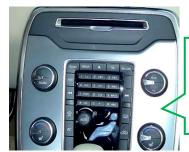
The EXIT or NAVI key or empty key below RADIO can be used to switch the interface.
