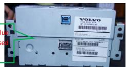
This interface can insert RGB + 2AV and 1 reverse camera video into the 2014 Volvo screens, the following are the features.
