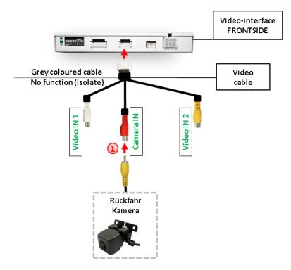
1 Connect the video-RCA of the after-market rear-view camera to the female RCA port of the video-interface which is labeled as CAM.
