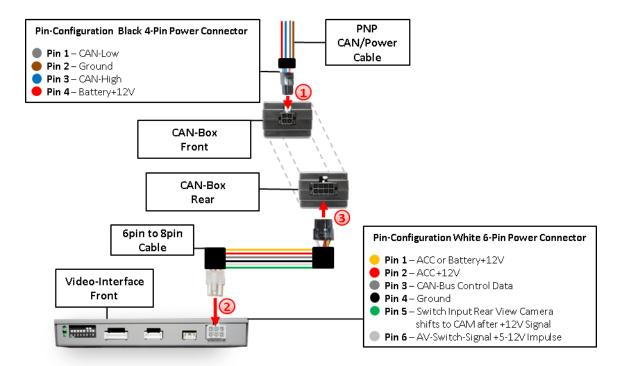
Connect the black female 8pin connector of the PNP Power/CAN harness to the male 8pin connector of the CAN-box.
