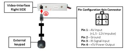
Connect the female 4pin connector of the keypad to the male 4pin connector of the video-interface.
