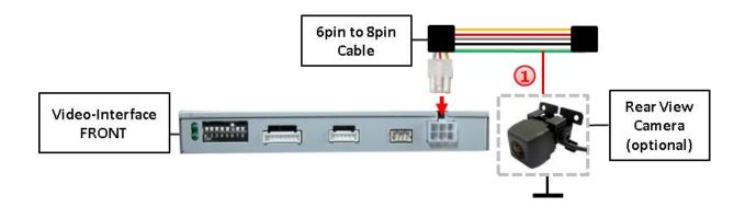
Additionally, the +12V (max. 500mA) power supply for the rear-view camera can be taken from the green wire of the 6pin to 12pin cable.
