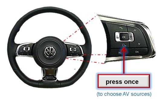
A press of the steering wheels voice key switches the input from factory mode to the inserted video sources. If - by dip switch setting - all inputs are enabled, the order is the following:
