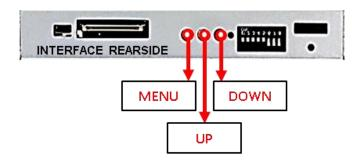
The picture settings are adjusted by the 3 buttons on the video-interface. Press the MENU button to open the OSD settings menu. To switch to the next menu item, pressing UP and DOWN will change the selected value. The buttons are embedded in the housing to avoid accidental changes during or after installation. The picture settings have to be done separately for AV1 and AV2 while the corresponding input is selected and visible on the monitor.
