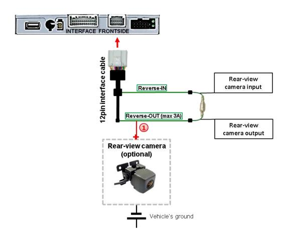
The 12 V power supply for the rear-view camera (max 3A) has to be taken from the green wire "Reverse-OUT" of the 12pin interface cable to avoid an unnecessary, permanent power supply to the camera electronic.
