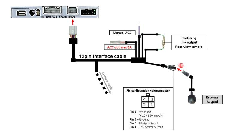
Connect the keypad's female 4pin connector to the 12pin interface cable's male 4pin connector.
