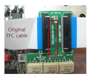
Connect Original FFC cable to sub-board.(LCD-OUT(BOTTOM))
