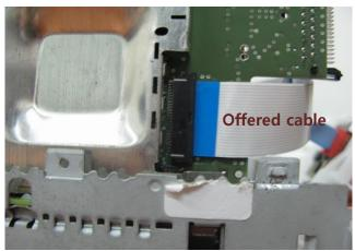
Connect offered FFC cable to sub-board.(LCD-IN (BOTTOM))
