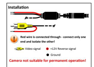
**Note:** If the camera is powered by reverse signal we recommend to install a relay between power supply of reverse signal and power supply of the camera to ensure a stable and uninterrupted power supply and avoid unwanted errors in the board computer.
