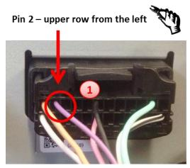
1 Cut the cable at pin 2 of the upper row from the left side and isolate both ends.
