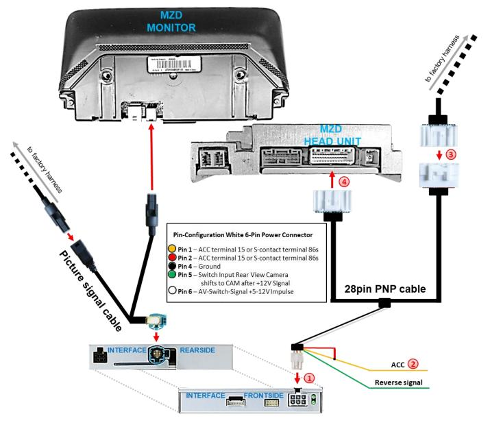
(1) Connect the 6pin cable's white female 6pin pin connector to the male 6pin connector of the video interface.
