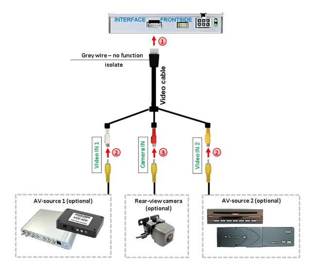
Connect the video cable's female 6pin connector to the video interface's male 6pin connector.
