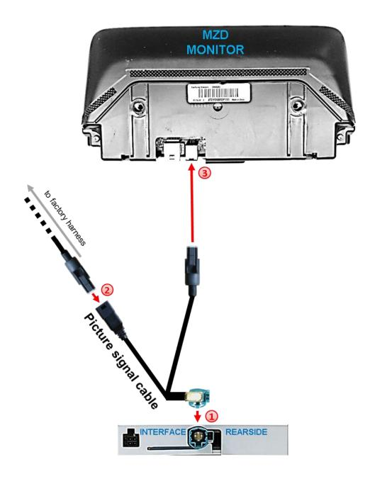
Connect the enclosed picture signal cable's female waterblue coloured HSD+2 connector to the male waterblue coloured HSD+2 connector of the video interface.
