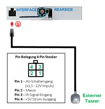
Connect the keypad's female 4pin connector to the video-interface's male 4pin connector.
