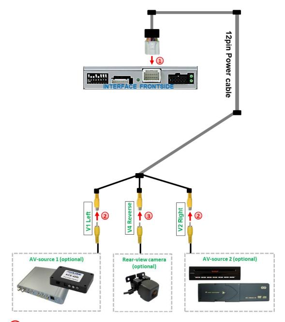
Connect the 12pin interface cable's female 12pin connector to the interface's male 12pin connector.
