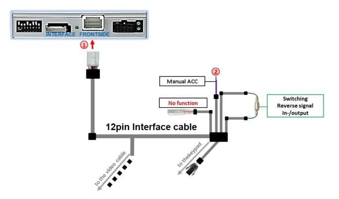
(1) Connect the female 12pin connector of the 12pin interface cable to the male 12pin connector of the video interface.
